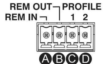
**C** “PROFILE 1” – Using a toggle switch with a latched ground signal to this point or in combination with “Profile 2” allows users to toggle between the DSP’s 4 user defined presets without the need of a controller or PC.
