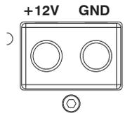
“GND” – Connect your amplifier with this terminal to the vehicles ground. The ground wire should be connected directly to the chassis of your vehicle via a 4 Gauge OFC ground cable. Find a clear location close to the amplifier and remove all paint and/or sound deadening. Use a #10 or larger screw to secure it. Never use a seat or seat belt bolt for grounding.
